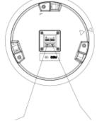
Red wire clamp is for positive pole. Black wire clamp is for negative pole.
