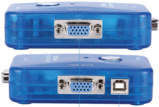
VGA output interface USB interface
